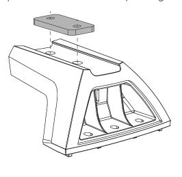
From the LockNLoad leg kit, assemble 1 x M8 spring washer and 1 x M8 washer onto each M8 set screw 16 mm in the order shown.
